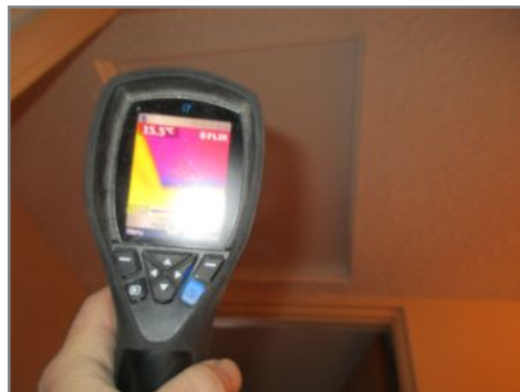
Thermal imaging shows heat loss at attic hatch
